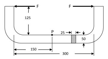
a. (5 pts) Find the endurance limit for the bar material assuming a machined finish, operating temperature below 125F, and 99% reliability.
