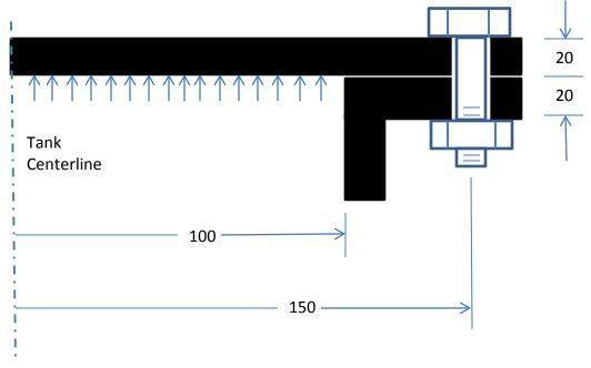
a. (5 pts) The bolts are initially tightened to 80% of their proof strength. Find the initial tension in each bolt.
