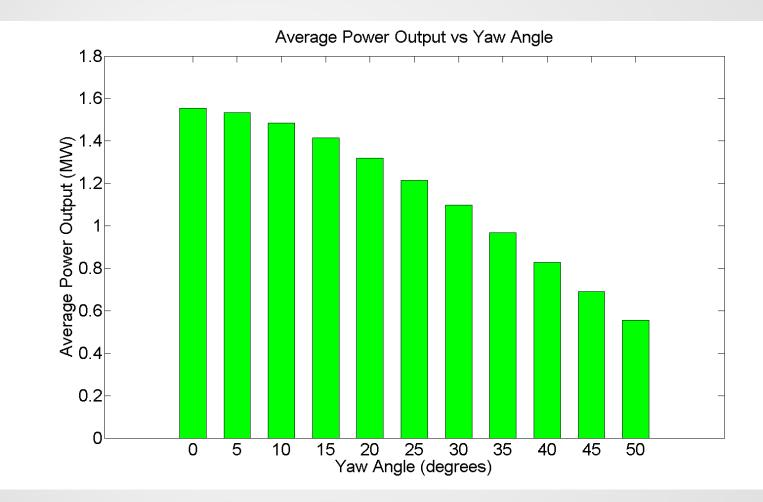
While yawing a wind turbine will deflect and reduce the intensity of its wake, it will also reduce its power output
