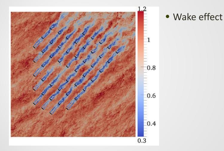
Churchfield, M., et al. *A Large-Eddy Simulation of Wind-Plant Aerodynamics*. National Renewable Energy Laboratory.
