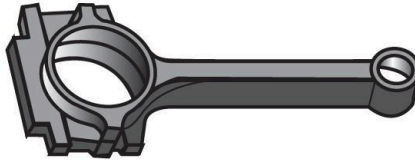
Figure 3: A connection rod (including the bottom bearing cap). The overall dimensions are approximately 150 mm in length, 50 mm in width, and 25 mm in depth.
